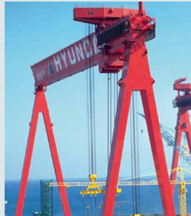
Single girder construction 900 t / 140 m
